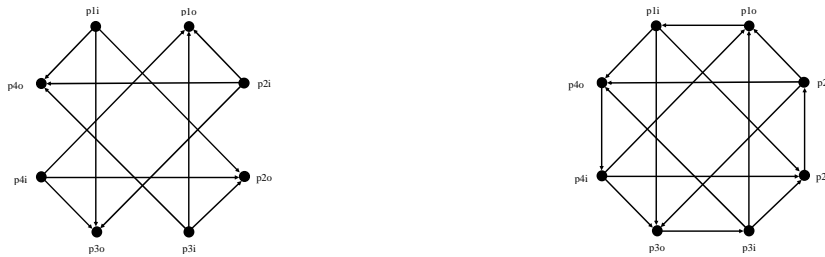
a) without terminal devices ( n2s1 ) b) with attached terminal devices ( nf2s1 ) Figure 4 – The transmission graph of a communication device
